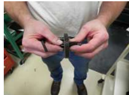
While most gears produced at Forest City Gear are metal, the company also machines various thermoplastic and composite materials, such as this helical plastic gear.
