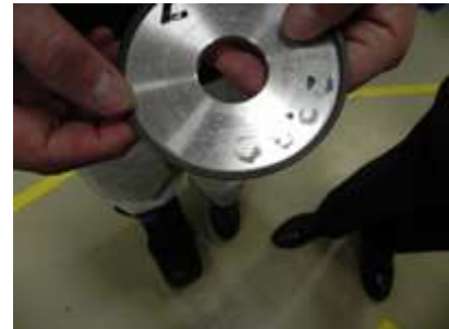
Diamond grinding wheels are used to keep the cutting tools and gear hobs in optimum condition.
