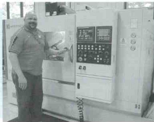
Employee training is a high priority at Forest City Gear, as the company continually invests in a wide variety of new equipment. Blanking Supervisor Tommy Kalt shows off a new CNC lathe that makes gear blanks.
